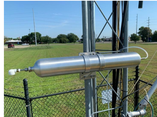
Buffered intake, rain cap and 3l buffer volume
